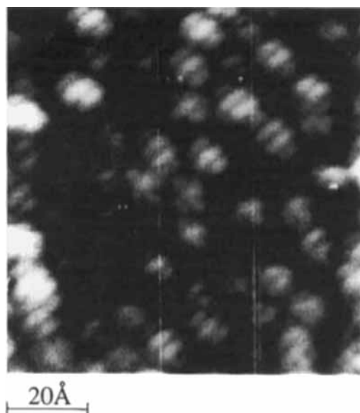
Figure 3 STM image of the first layer of the C_{60} molecules. The image shows some internal structure (three or four rows running in parallel) for the individual C_{60} molecules. Similar internal structures were also observed for the C_{60} adsorbed on the Si(111) c(7 \times 7) surface. Figure reproduced from Ref. 25.
